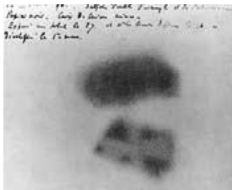
Figure 1: One of Becquerel's photographic plates fogged by exposure to radiation from potassium uranyl sulfate. The shadow of a metal Maltese Cross placed between the plate and the uranium salt is visible.
